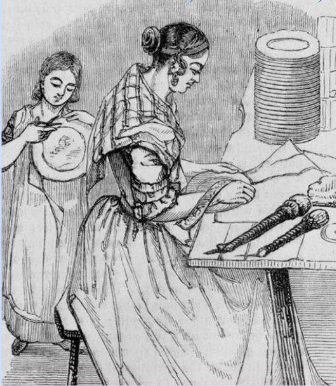
Transferrers working in a 19th Century pottery. (Drawing courtesy of Spode Museum Trust.)
